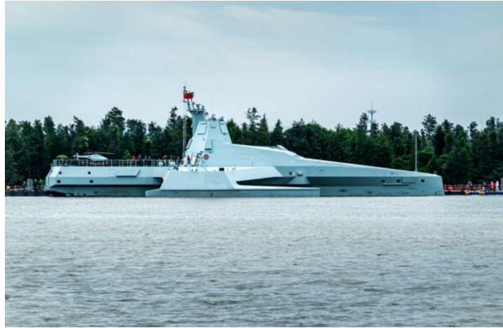
Figura 12. Buque no tripulado “Orca” de PLAN. Fuente: Rahmat, R. (2024). Airshow China 2024_ China debuts 500 tonne unmanned surface vessel. JANES. https://www.janes.com/osint-insights/defence-news/security/airshow-china-2024-china-debuts-500-tonne-unmanned-surface-vessel
